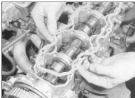
8.29a Fitting a new camshaft cover gasket
