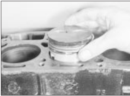
15.11 Offering the piston to the bore
