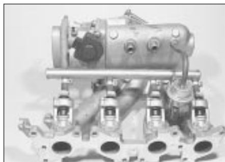
13.11b Inlet manifold showing injectors fuel rail and associated components
