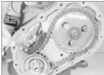
14.20 Fitting a new timing cover gasket
