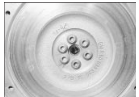
16.4 Flywheel retaining bolts are socket-headed
