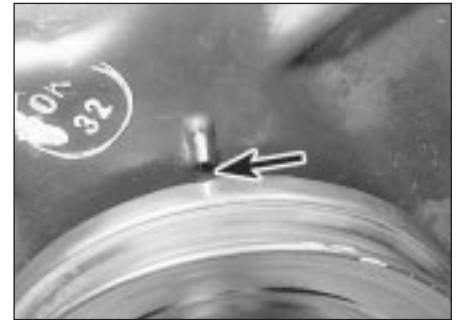
7.7 Ignition timing marks (arrowed) in alignment
