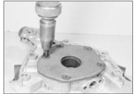
14.1 Using an impact screwdriver to undo the oil pump rear cover screws
