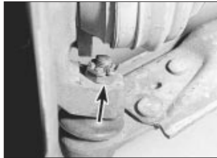
5.3 Control arm balljoint nut (arrowed)
