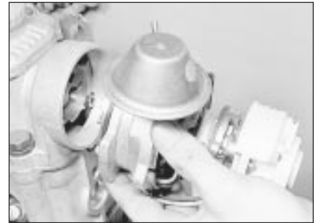
3.5 Removing the distributor from the camshaft housing
