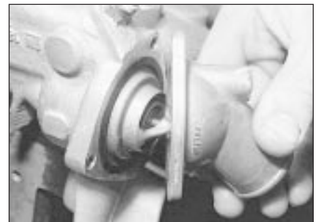
4.9a Removing the thermostat cover . . .
