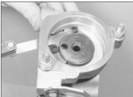
9.10 Checking the camshaft endfloat
