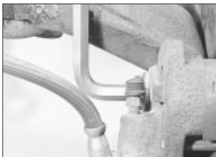
10.6b . . . then unscrew the caliper bolts . . .
