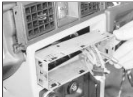
25.4 Removing the radio surround
