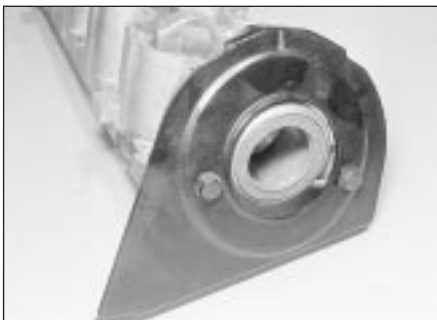
9.7 Camshaft belt cover backplate (1.3 litre engine shown)
