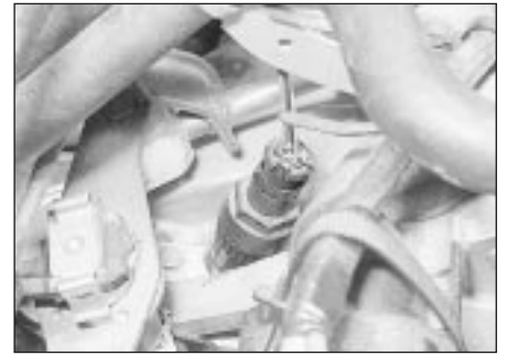
25.22 Speedometer sender (used with digital instrument panel)
