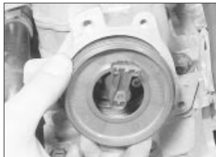
3.9 Extract the insulator
