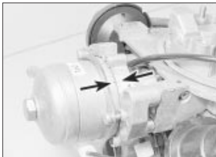
15.12 Choke cover alignment marks (arrowed)
