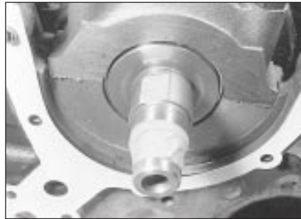
13.6 Tape the crankshaft nose
