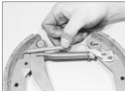
6.17b Fitting the upper return spring to the adjuster lever bracket
