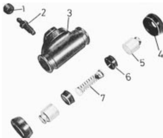
12.6 Exploded view of a rear wheel cylinder
