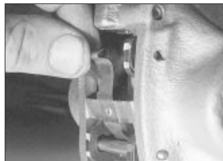
5.9b Hooking the spring under one retaining pin
