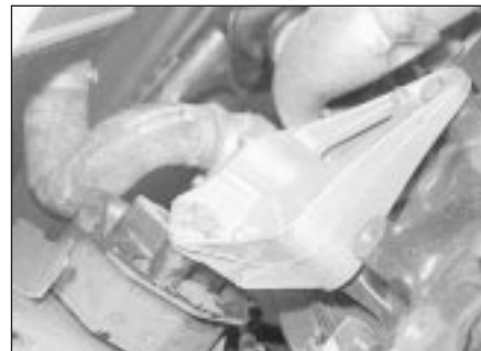
23.20b Engine/transmission right-hand mounting
