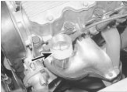
3.2a Hot air pick-up tube (arrowed) engages with air cleaner
