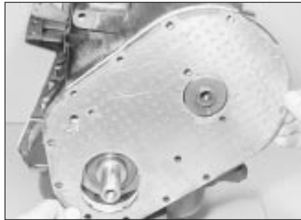
18.4b Removing the engine front plate
