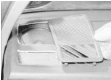
10.1 Removing an end grille and speaker
