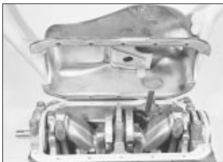
11.9 Refitting the sump
