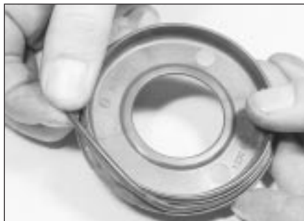
3.27 Renewing the insulator sealing ring
