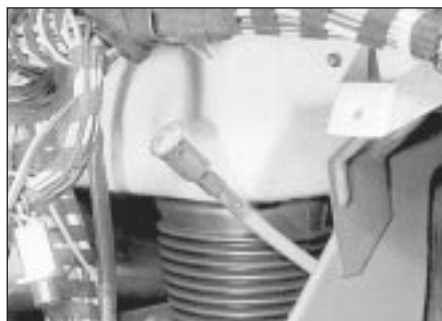
10.2 Speedometer cable at instrument panel end
