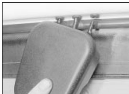
21.9 Removing the window-mounted motor
