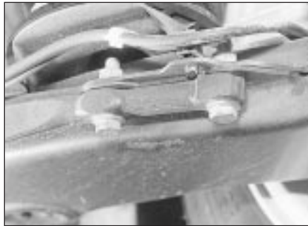
13.7 Auxiliary anti-roll bar mounting - 2.0 litre 16-valve models
