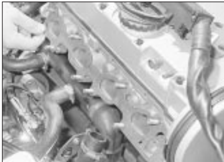
13.33 Fitting a new inlet manifold gasket
