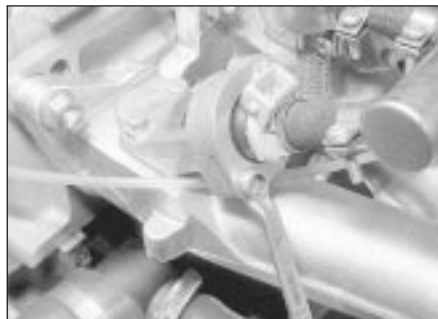
12.8 Undoing a fuel injector retaining bolt
