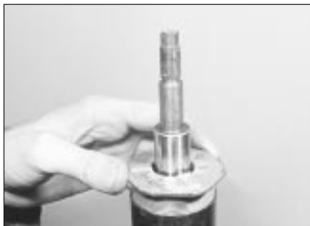
4.6b Removing the strut ring nut
