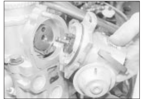
3.6e Removing the distributor - note peg-and-hole drive (1.6 litre carburettor model shown)
