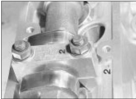
10.6 Matching numbers on bearing cap and cylinder head
