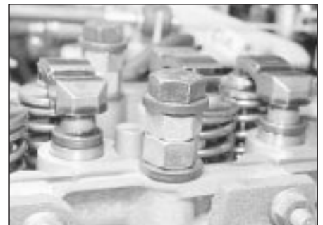
9.3 Cylinder head bolt, with washers and nuts for spacers, used to clamp head
