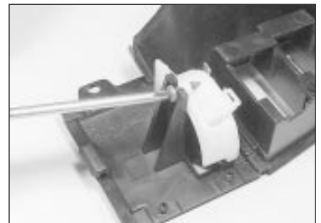
4.8 Removing the instrument illumination control
