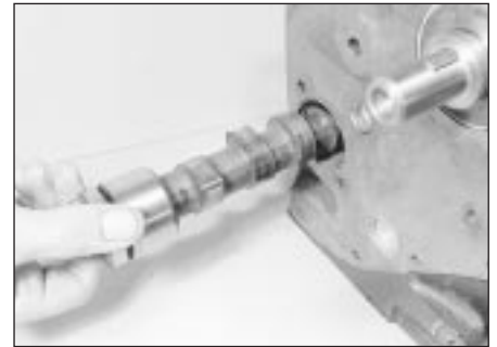
18.5 Removing the camshaft
