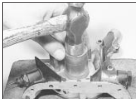
14.6 Fitting a new front oil seal
