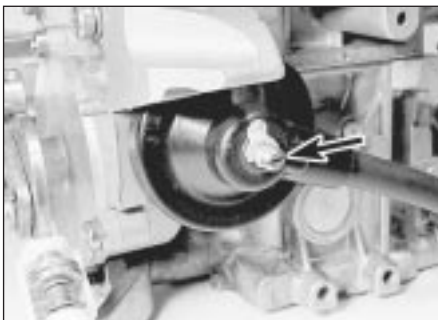
14.8a Choke valve gap adjustment screw (arrowed)
