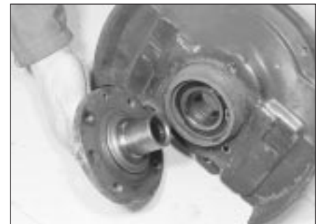
3.3b Hub removed from the carrier
