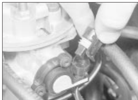
11.3a Detach the wiring connector from the throttle valve potentiometer
