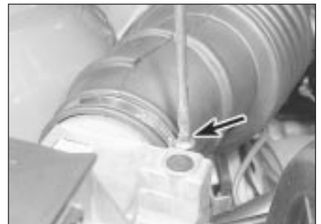
12.12 Disconnecting the airflow meter trunking
