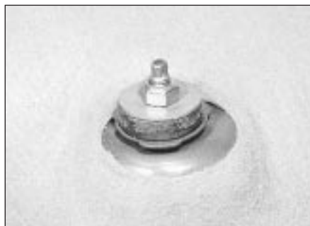
12.2 Rear shock absorber upper mounting - Hatchback
