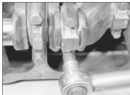
15.14b Tightening a big-end bearing cap bolt
