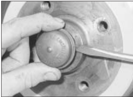
8.3 Levering off the grease cap
