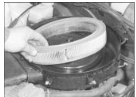
24.2b . . . and withdraw the filter element
