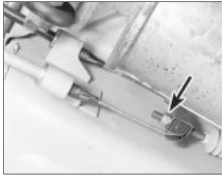
19.3 Handbrake cable adjusting nut (arrowed) on yoke - rear drum brake models
