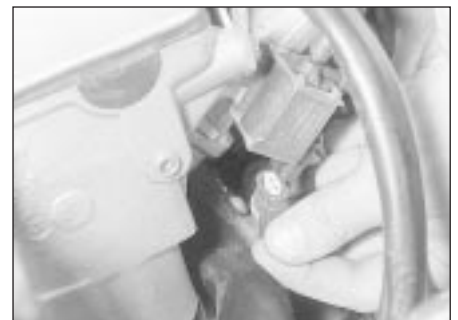
12.100 Disconnecting the vent valve multi-plug
