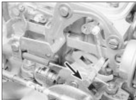
10.5 Choke cable inner clamp screw (arrowed)
