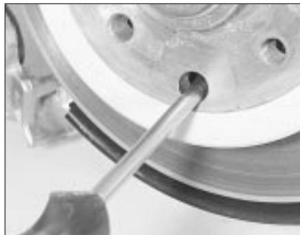
19.11b . . . and can be adjusted using a suitable screwdriver
