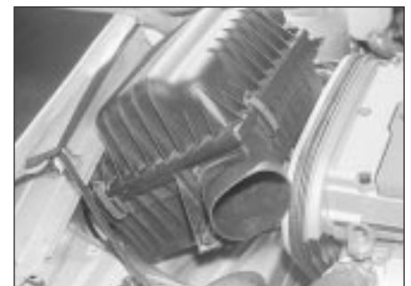
2.5c Removing the air cleaner - 2.0 litre 16-valve
