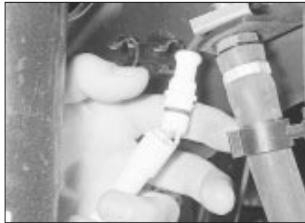
22.3b Separating a front sensor connector
