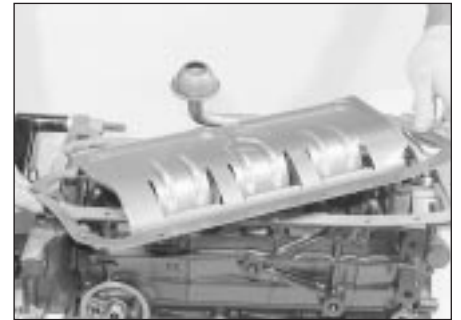
12.7a Removing the oil baffle plate. This model has two cork gaskets . . .
