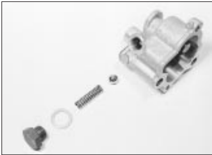
13.4 Oil pump and pressure relief valve components
