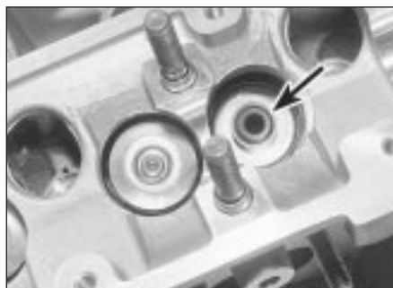
12.6d ... the valve stem oil seal (arrowed) ...
