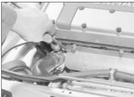
14.3 Removing an exhaust manifold heat shield bolt
