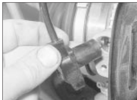
22.2c Removing a front wheel speed sensor
