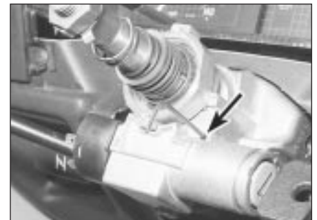
23.6 Releasing the steering lock detent spring with an Allen key (arrowed)
