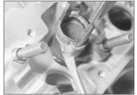
12.13 Fitting a valve collet
