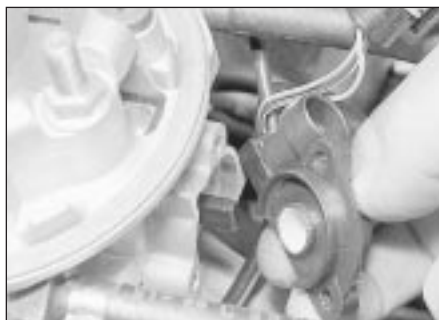
11.3b Throttle valve potentiometer removal
