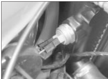
7.2 Cooling fan thermostatic switch screwed into side of radiator
