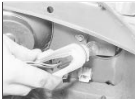
11.9 Removing a direction indicator bulb and holder
