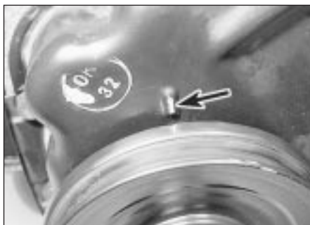
6.3 Ignition timing marks (arrowed) in alignment
