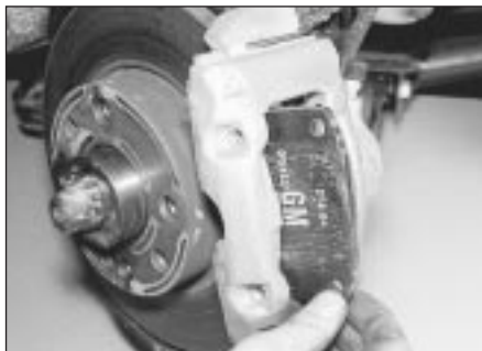
4.5 Removing the outboard pad
