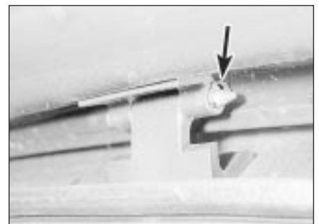
20.4 Tailgate hinge showing circlip (arrowed)
