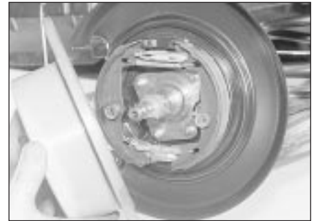
8.5 Removing the rear disc
