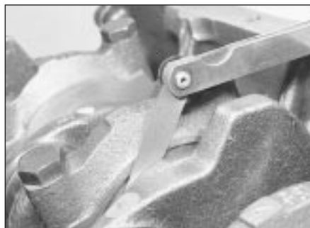
20.19 Checking crankshaft endfloat
