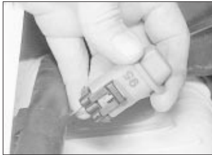
4.6 Octane rating plug in the "95" setting position
