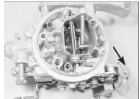
12.11b Choke valve gap adjusting screw (arrowed)
