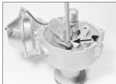
7.5 Undoing the condenser retaining screw
