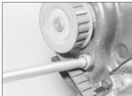
7.8 Slackening a water pump bolt
