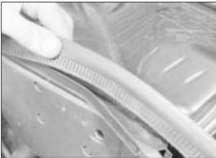
9.8a Lift the rubber seal to free the water
