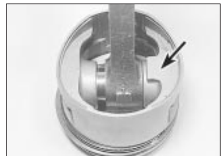
15.1 Large land (arrowed) faces the flywheel end of the engine
