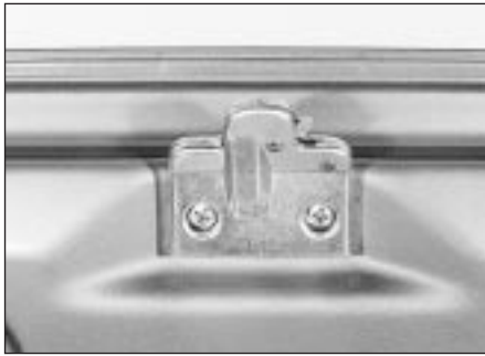
26.2 Boot lid lock securing screws
