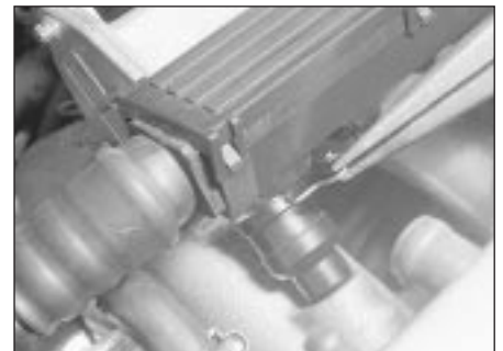
12.66a Removing the spring clip from an injector multi-plug
