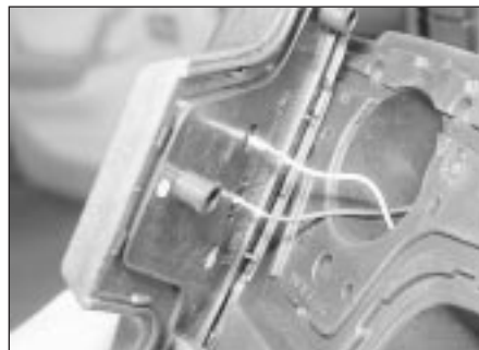
19.2 Removing the steering wheel central cap
