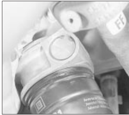
16.2 Circlip securing oil cooler thermostatic valve
