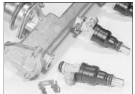
12.69b . . . and pull out the injector
