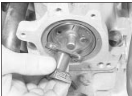
3.10b . . . and remove the rotor
