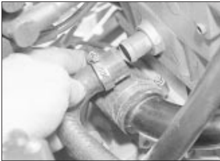
11.11 Disconnecting the heater hose from the cylinder head
