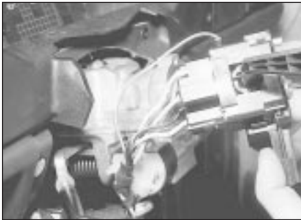
4.14a Drawing the steering column switches up the column
