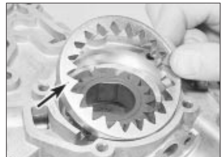
14.4 Gear outer face identification mark (arrowed)
