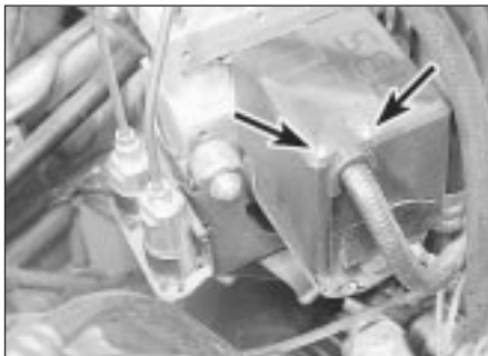
22.15 Two screws (arrowed) which secure the hydraulic unit cover
