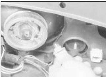
11.7 Removing a sidelamp bulb and holder
