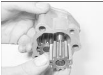
13.3a Removing the oil pump driving gear . . .
