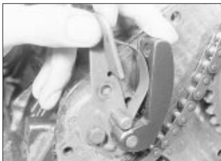
14.19a Fit the tensioner lower bolt . . .
