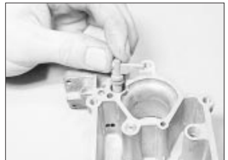
19.11 Removing the fuel discharge nozzle
