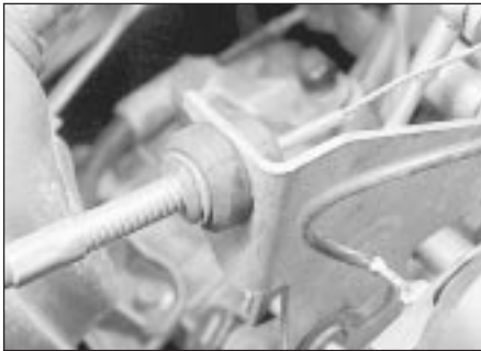
8.3 Accelerator cable bracket and bush
