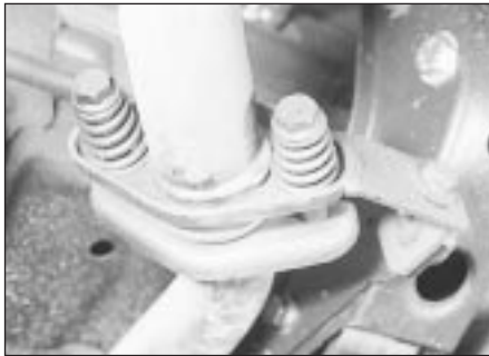
27.4a Exhaust system flexible joint
