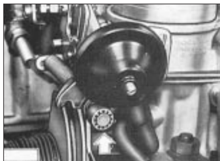
13.2 Fast idle adjustment screw (arrowed)
