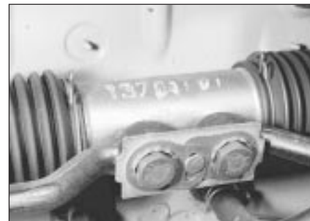
27.4 Tie-rod connection to steering rack
