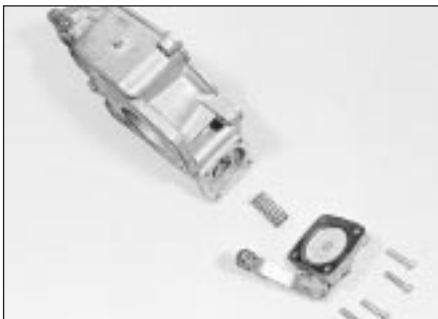
19.9 Accelerator pump components
