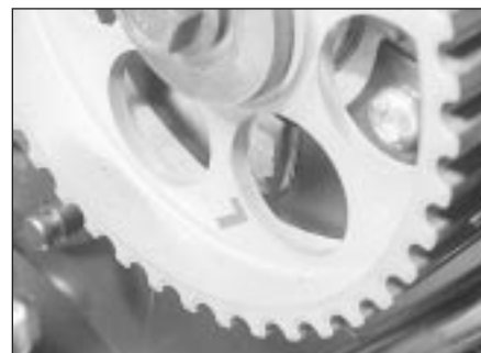
10.4 Exhaust camshaft sprocket is marked 'L'
