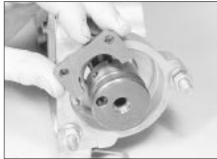
9.5b Removing the camshaft thrust plate
