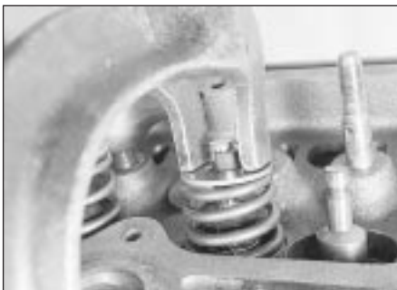
9.20 Compress the spring and fit the collets
